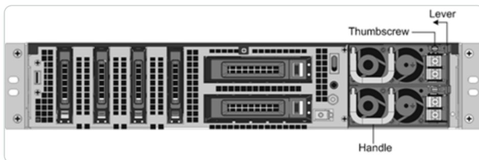
Figure 2. Remove the existing DC power supply
